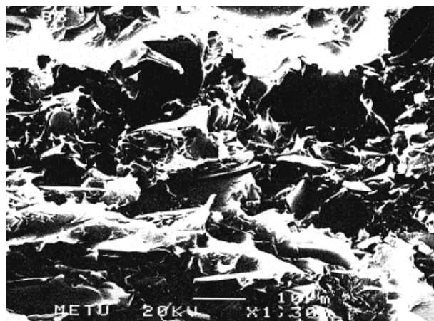
Figure 12 Fractograph of 15% perlite-filled 100-kGy-irradiated PP.
